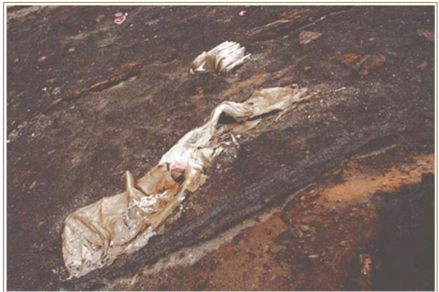
Both fire shelters had been removed from their packs. One of the shelters (top) was still "accordion" folded in the same shape in which it was packaged—indicating it had not been unfolded prior to burnover. The second shelter (bottom) had been partially unfolded before the burnover.
