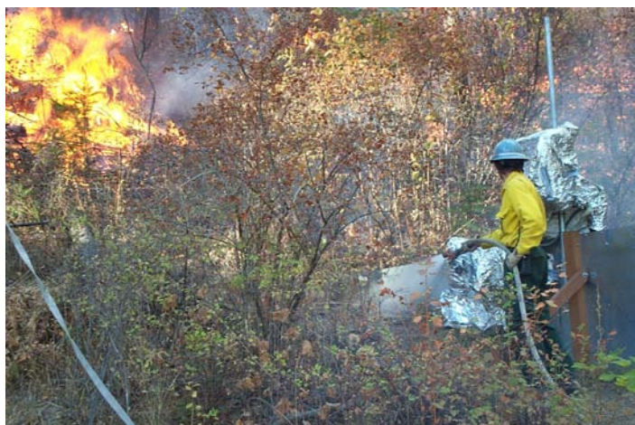
Figure 6. Protecting the instrumentation with fire blankets and water during the simulated wildfire at the Priest River Experimental Forest in October 2006.
