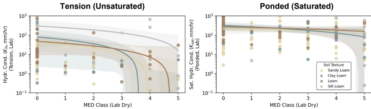
Figure 13 Tension (A) and Ponded Head (B) infiltration values using the cumulative infiltration method plotted against the sample MED value grouped by soil textural class. Note log scale on y-axis.
