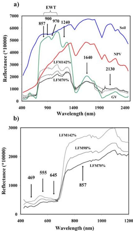
Figure 2) AVIRIS spectra of chamise with three LFM amounts. Wavelength regions used to calculate the various indices are labeled.
