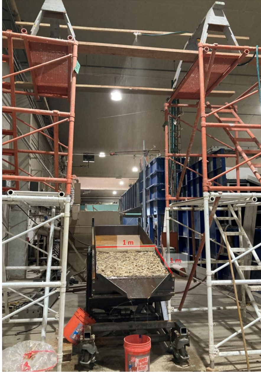
Figure 3. Flume setup with mulched soil filling the lower 1 m length of the tilt table.
