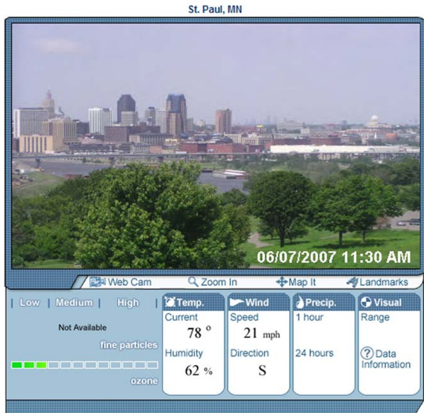
Figure 8 —St Paul, MN, “haze cam” image showing “current conditions. The live image is updated every 15 minutes. Visual range, measured by nephelometer, has been reported with the met data beneath the picture on many haze cam sites.
