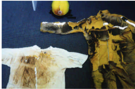
Figure 10 —Damage to personal protective clothing from Firefighter C (who received the most serious burn injuries), including Nomex coveralls, cotton T-shirt and fibreglass helmet.
