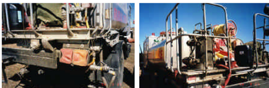
Figure 5 —Damage to the fire appliance, including tail lights, foam proportioner, pump cover and rubber hose fittings.
