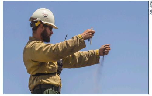
Measuring wind speed. Wind is a weather variable that can turn an ember into a wildfire. Knowing the wind direction and speed allows fire managers to effectively deploy resources or pull firefighters back from the line.
