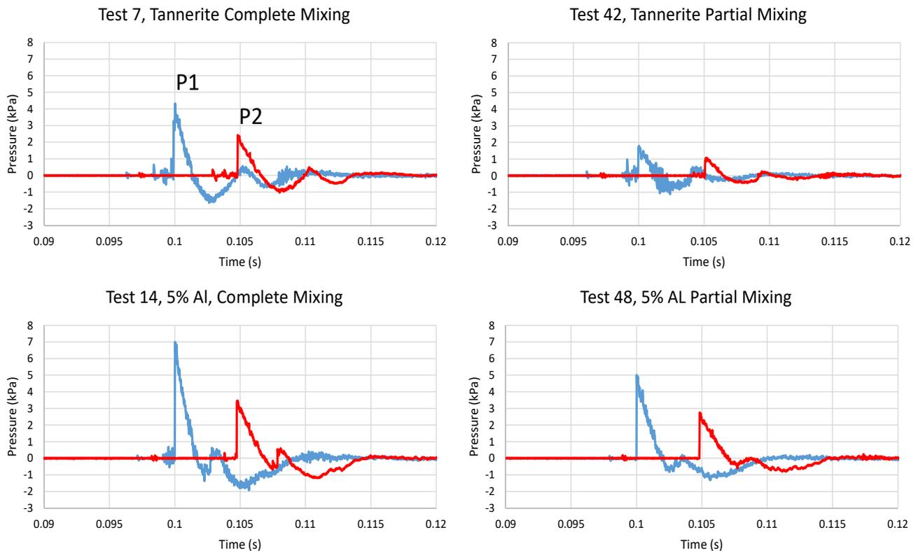
**Figure 14**—Graphs of air pressure perturbation from selected 2018 tests of exploding targets. All targets are 1 lb. Probe 1 (P1, blue) was 8 ft from the target. Probe 2 (P2, red) was 15 ft from the target (see also figure 1). Higher overpressure occurred with additional aluminum. Partial mixing diminished peak overpressure compared to complete mixing.
