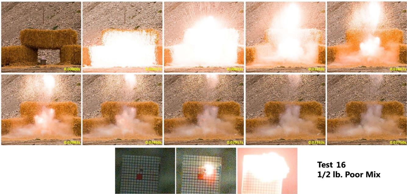
**Figure 11**—Sequence of images from test 16, 2015, showing large region of luminous burning and bright aluminum ejected from an incompletely mixed target. No ignition resulted.
