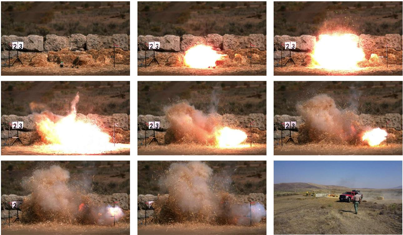
**Figure 7**—Test 23, 2018, 10 percent aluminum, partially mixed. Series showing explosion, vertical and lateral ejection of burning aluminum, residual combustion within the blast zone, and ignition of straw bales.
