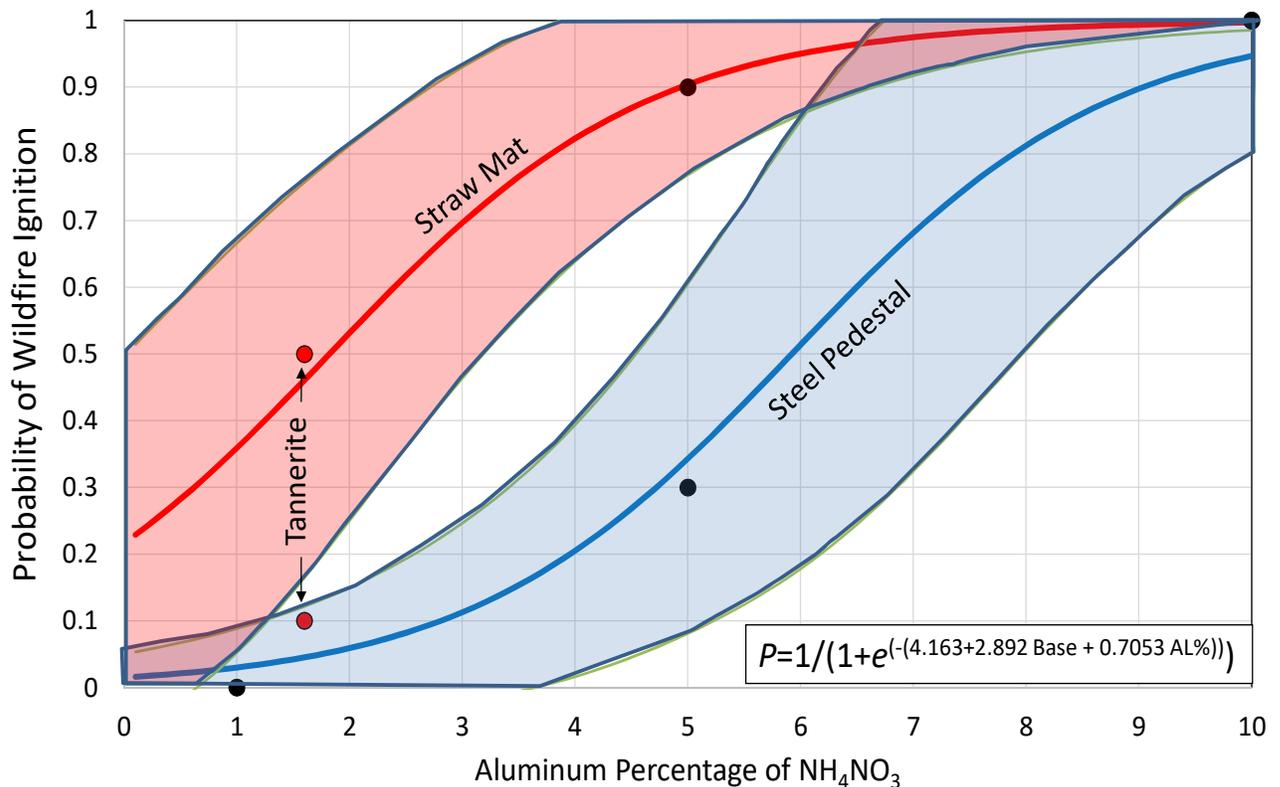
**Figure 9**—Logistic regression model and 95-percent confidence intervals from the 2018 tests relating the probability of wildfire ignition to the aluminum (AL) percentage of the aluminum-ammonium nitrate mass and the base material supporting the exploding target. Data points are averages of the 2018 data for these combinations. Logistic model uses predictors of base = 0 for pedestal and 1 for straw. Model had residual deviance of 40.31 and Akaike Information Criterion of 46.31.
