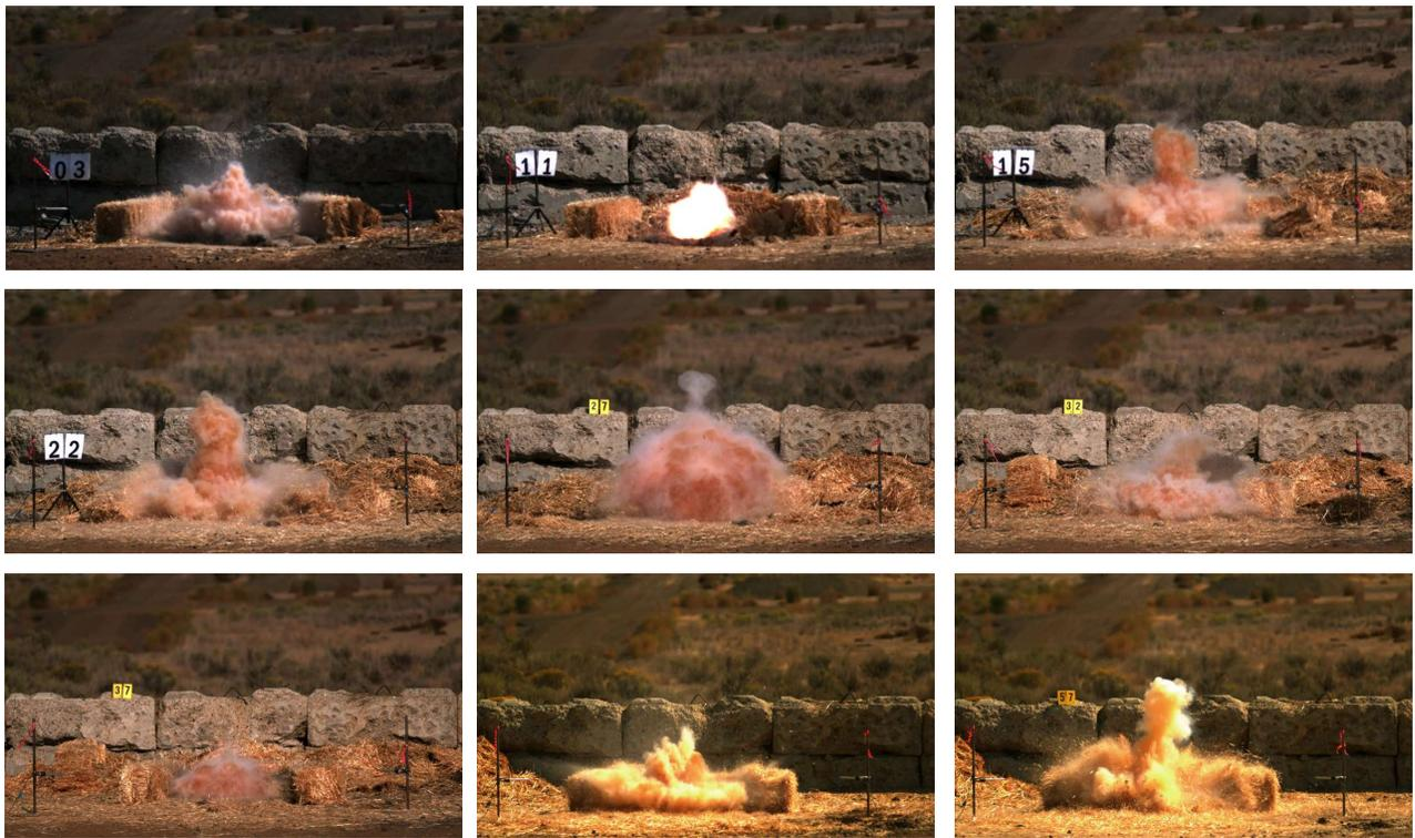
**Figure 12**—Frames from selected 2018 tests showing smaller explosion envelope with little visible burning within the blast volume or burning aluminum particles. Number seen in the photograph is the test number corresponding to those in Appendix 2.
