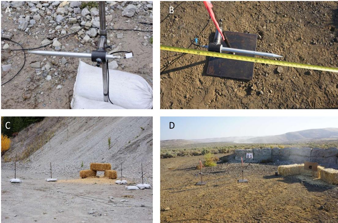
**Figure 6**—Setup of pressure probes used to measure the blast pressure from the exploding targets for (A) 2015 tests (close-up), (B) 2018 tests (close-up), (C) 2015 tests, and (D) 2018 tests. See also figure 1.
