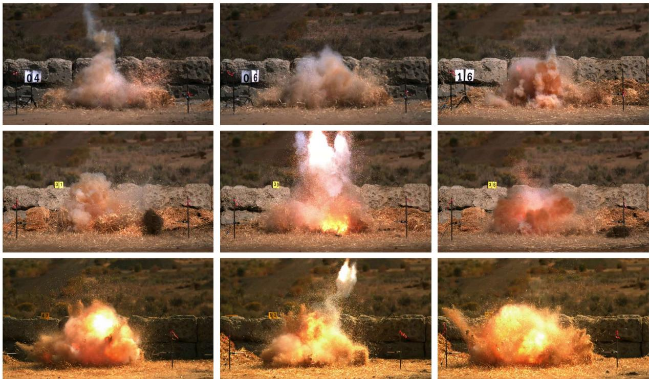
**Figure 10**—Frames from selected 2018 tests showing ejection of burning aluminum from blast (bright colored sparks) and burning within the blast volume. Number seen in the photograph is the test number corresponding to those in Appendix 2.
