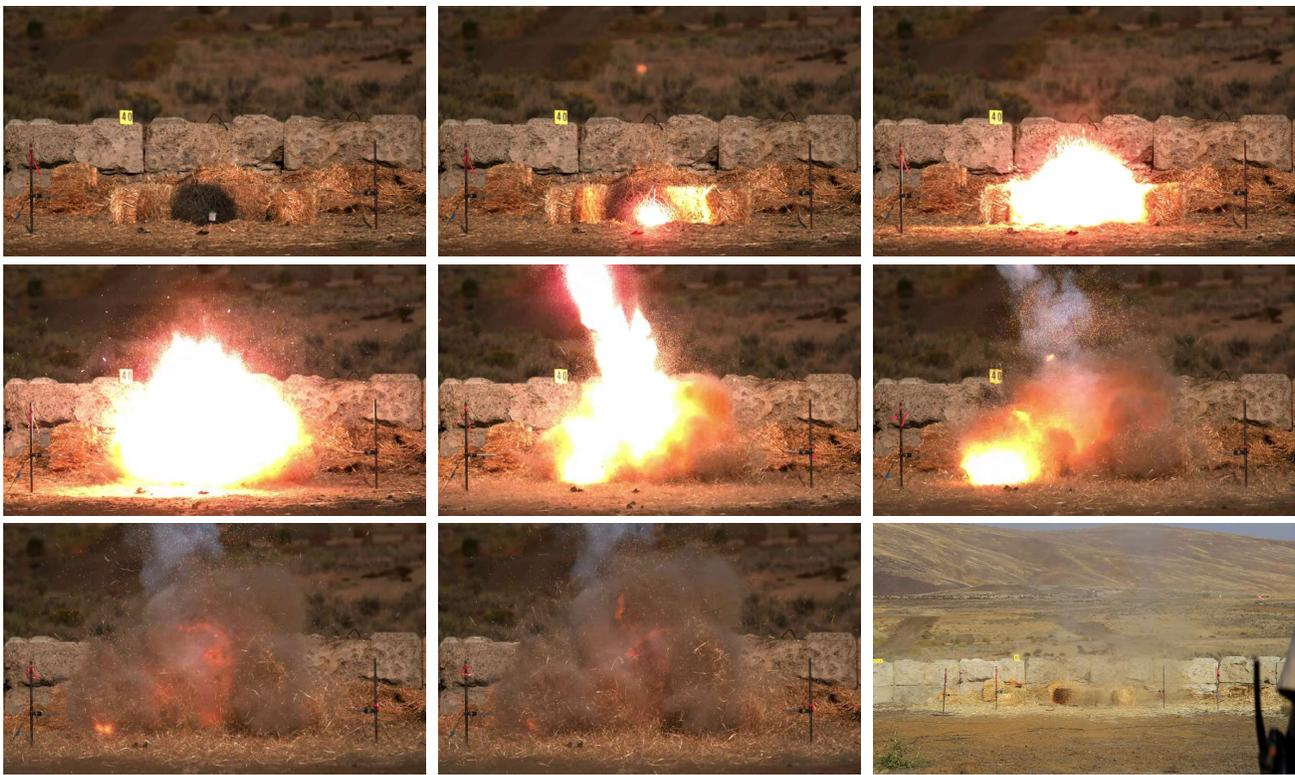
**Figure 8**—Test 40, 2018, 10 percent aluminum, partially mixed. Series showing explosion, vertical and lateral ejection of burning aluminum, residual combustion within the blast zone, and ignition of straw bales.
