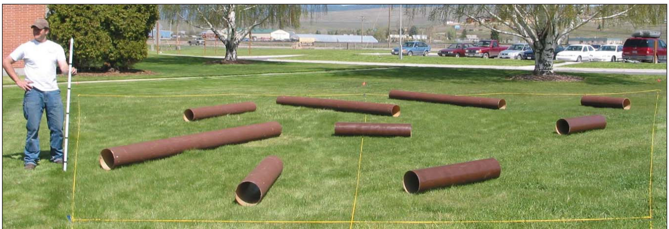
Figure 4 —A picture showing the 30 cm diameter brown tubing cut at various lengths and put on the 100 \text{ m}^2 plot to approximate a loading.
