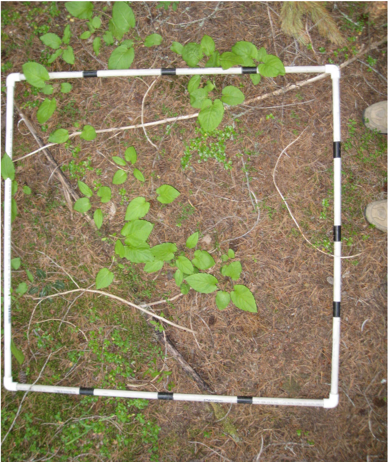
Figure 7 —A 1 m x 1 m square plot sampling frame to be used to outline the photo to emphasize fuel conditions and set the spatial boundary of fuel estimates. Note the frame is made of 2.5 cm (1 in) diameter white PVC pipe and black tape is used to identify half and quarter portions within the frame to aid in visual estimation. The inside of the frame delineates the 1 m 2 area.
