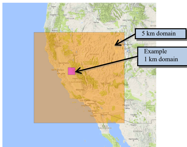
Figure 1: Mesoscale model domains used by FireBuster. The 5-km domain covers all of the state of California (and Nevada as well). Forecasts for the 5-km domain are run twice daily. The 1-km domain forecasts can be run when needed for specific areas.
