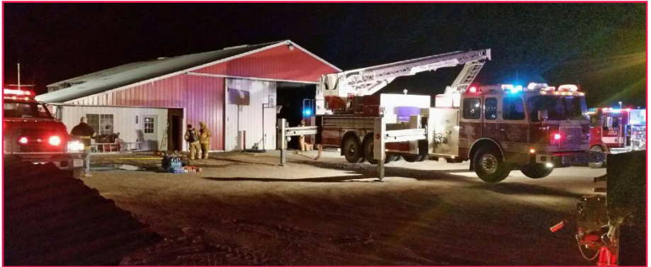
Mead Volunteer Fire and Rescue Department HEMMTs in action. Standard size for these heavy-duty vehicles is over 30 feet (9.1 m) long, 8 feet (2.4 m) wide, and 9 feet (2.7 m) high. Photo: Nick Raver, Mead Volunteer Fire and Rescue Department.
