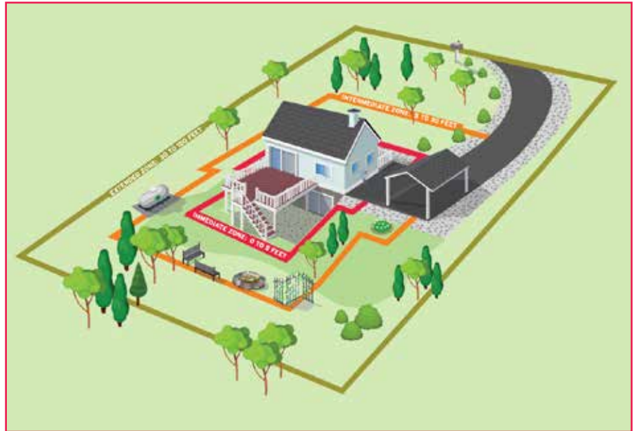
Figure 1 —The three home ignition zones (0–5 feet [0–1.5 m], 5–30 feet [1.5–9 m], 30–100 feet [9–30 m]). Reducing risks within the three zones increases the chances of a home surviving a wildfire. Source: National Fire Protection Association.
