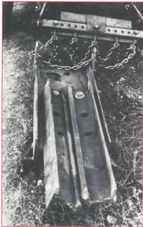
◀ Figure 4 —Top view of the plow showing how two 36-inch (91-cm) railroad rails can be bolted for the most efficient plowing. Photo: Stephen Arno, Intermountain Research Station, Missoula, MT, 1994.
