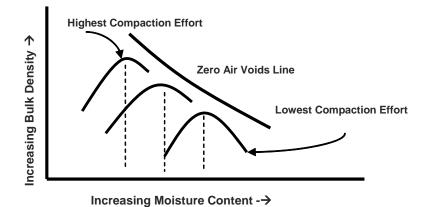
Figure 1: General relationships between moisture content, compaction effort and maximum bulk density [13].
