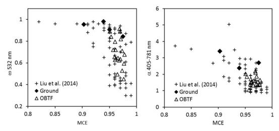
Fig. 2. Single scattering albedo ( $\omega$ ) at 532 nm and absorption angstrom exponent ( $\alpha$ ) for 405–781 nm for burn averaged values. "Ground" CO measurements for MCE are 2 min samples and may not be reflective of the whole burn. Liu et al. (2014) measurements are for wheat and a variety of grass species.
