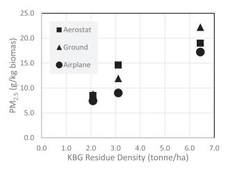
Fig. 6. Effect of KBG crop residue density (dry weight) on PM2.5 emission factors across all platforms. PM from field B and LL were gathered on the same sample media.
