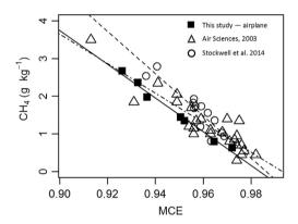
**Fig. 5.** Methane (CH<sub>4</sub>) emission factors as a function of MCE for fire average values measured in this study from the airplane platform (Solid line, slope =  $-44.9~(\pm 2.5)$ ,  $R^2=0.98$ ) and from literature (dashed line, slope =  $-56.2~(\pm 7.5)$ ,  $R^2=0.84~(Stockwell$  et al., 2014b), and dash-dot line, slope =  $-39.3~(\pm 3.9)$ ,  $R^2=0.81$ , Air Sciences Inc (2003).
