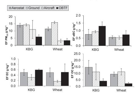
Fig. 1. Average PM<sub>2.5</sub>, EC, eBC, and OC emission factors. Bars indicate ±1 standard deviation (std.).
