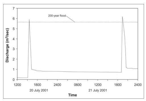
Figure 6—Storm hydrographs from Laird Creek, near Sula, Montana. Adapted from data from the U.S. Geological Survey.
