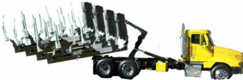
Hooklift-equipped truck delivers bunks
