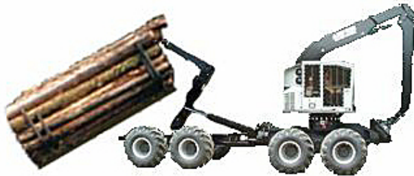
Forwarder sets a loaded bunk at roadside
