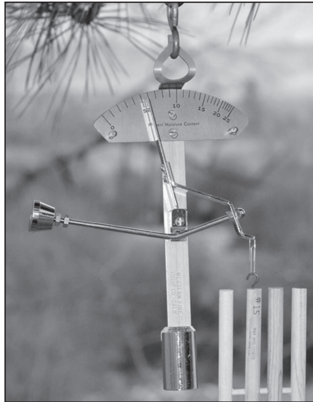
Portable scales, developed by Harry Gisborne and his colleagues, were used for weighing ponderosa pine moisture indicator sticks in the field (photo: USDA Forest Service).
