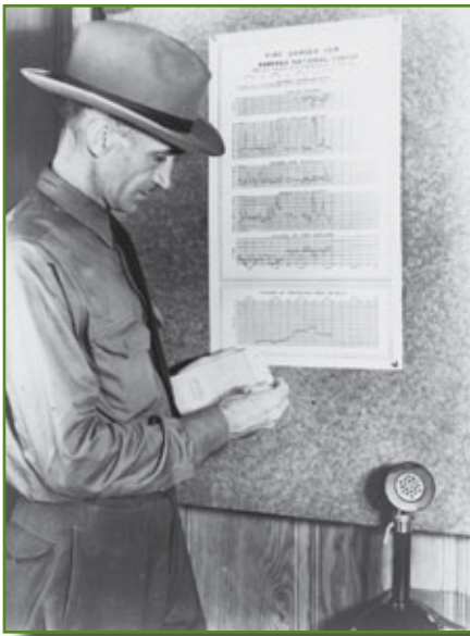
Harry Gisborne uses an early fire danger meter to predict forest fire activity in the Kaniksu National Forest in 1937 (photo: courtesy of the Forest History Society, Durham, NC).
