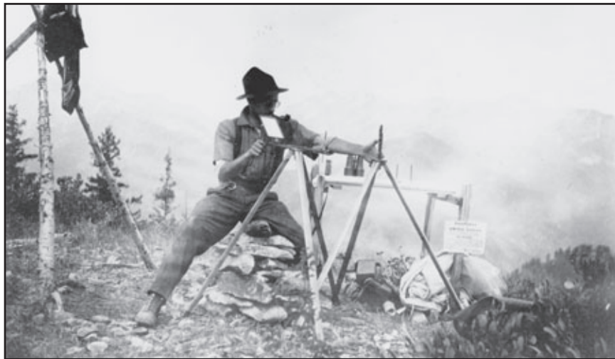
Harry T. Gisborne operating a double tripod heliograph, Tip Top Lookout, Wenatchee National Forest, Washington, 1915 (photo: courtesy of the Forest History Society, Durham, NC).
