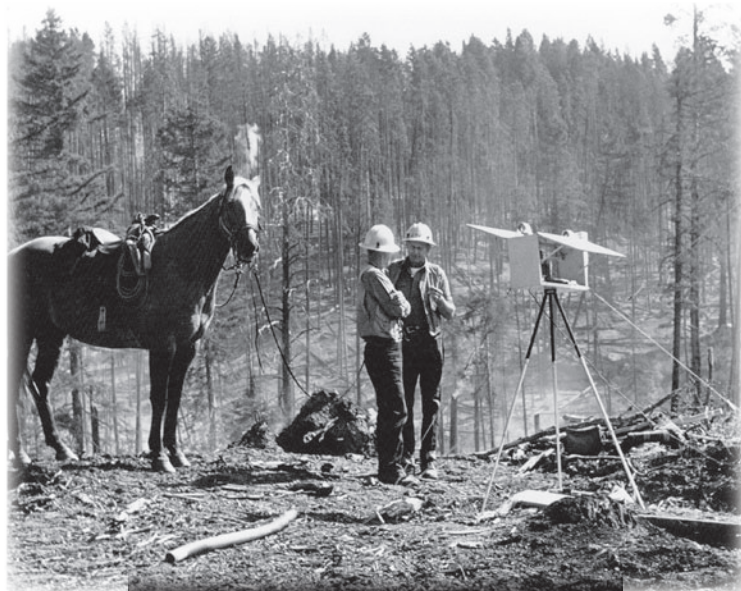
Using a portable weather station to gather fire weather data during the 1959 Brackett Creek Fire in the Gallatin National Forest (photo: USDA Forest Service).
