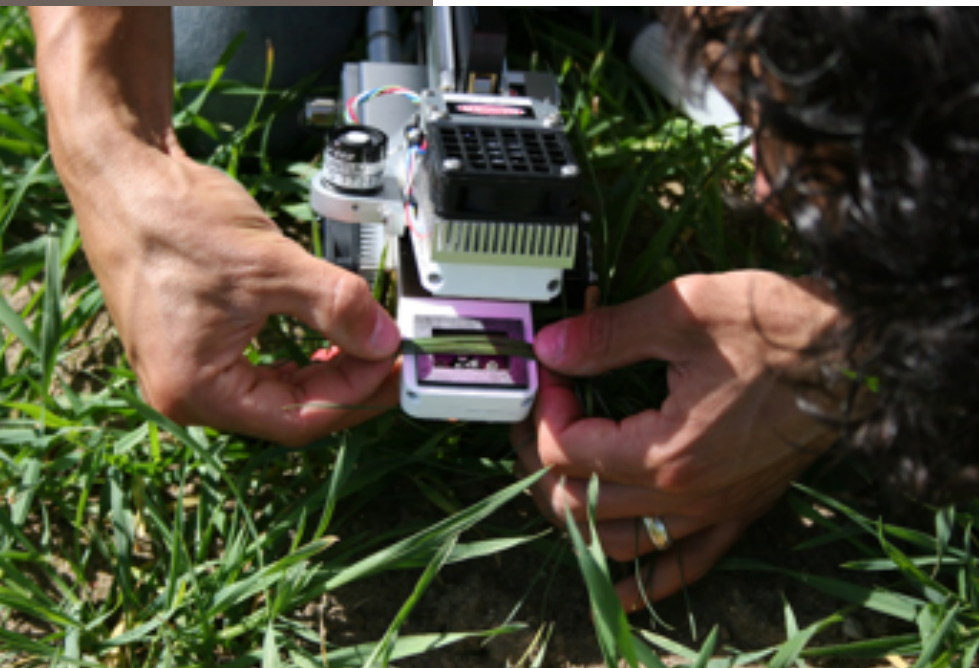
Measuring gas exchange on an establishing seedling.
