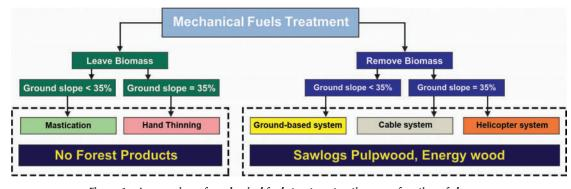
Figure 1-An overview of mechanical fuels treatment options as a function of slope.
